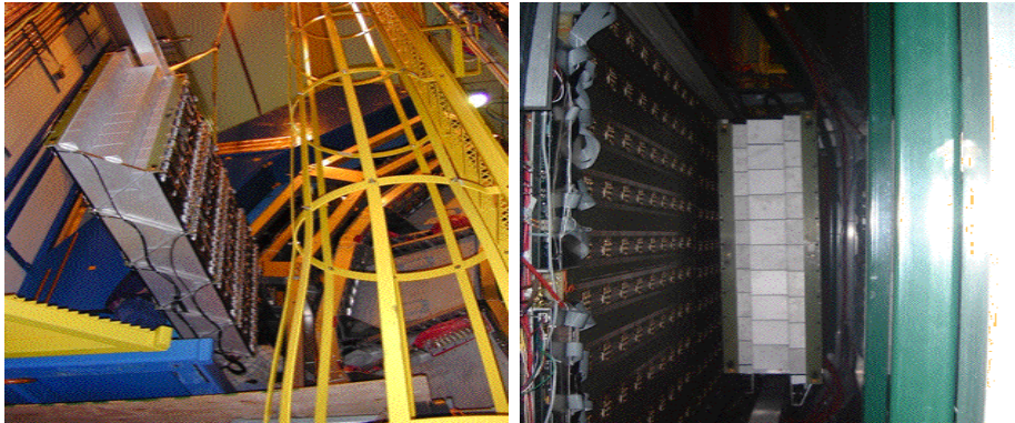
Figure 2.15: Installation of Aerogel Cherenkov Counter.
