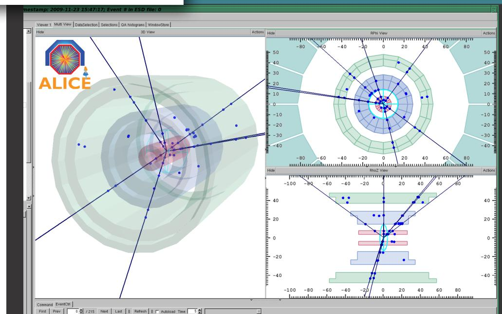
(3D view,  $r-\phi$  and  $r-z$  projections), the dimensions are shown in cm. The dots correspond to hits in the silicon vertex detectors (SPD, SDD and SSD), the lines correspond to tracks reconstructed using loose quality cuts.
