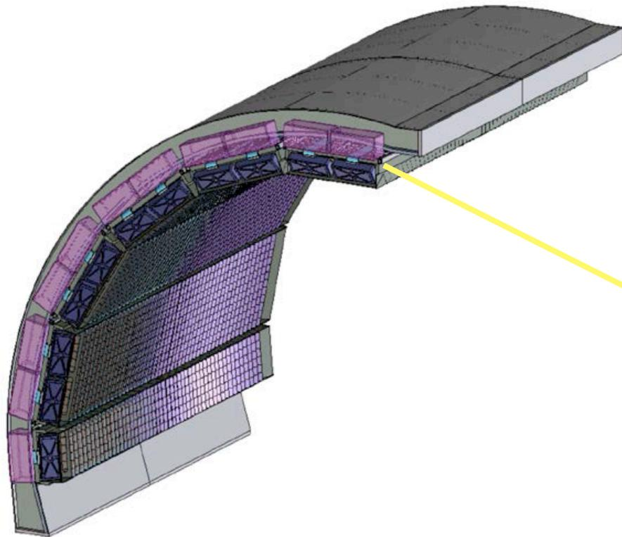
Lead-Scintillator Sampling Calorimeter
